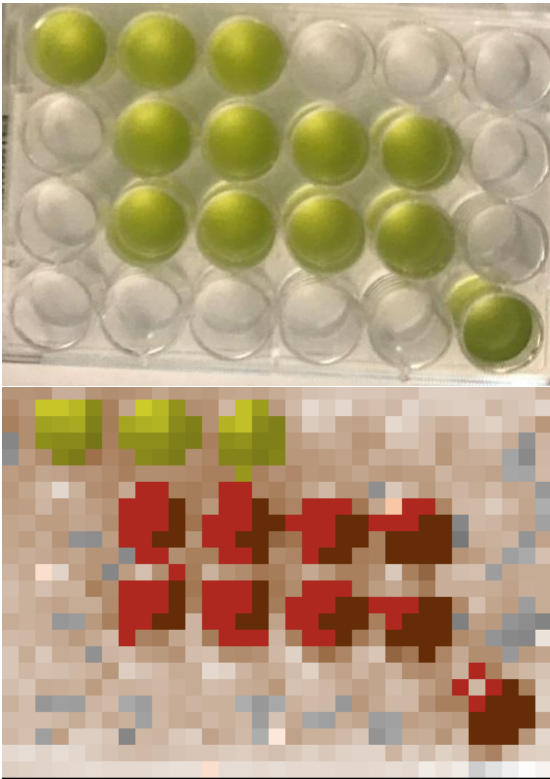
Figure 5. These pictures show the original pictures of the algae and the pictures of the algae after it has been analyzed. Wells B2, B3, and B4 have 8 PPT of salt. Wells C2, C3, and C4 have 32 PPT of salt. Wells B5, C5, and D6 have 64 PPT of salt.
