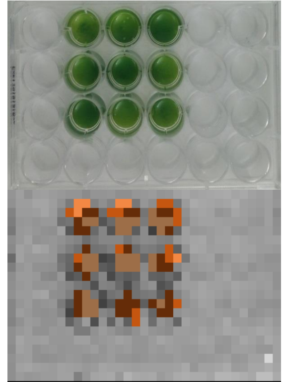
Figure 7. These pictures show the original pictures of the algae and the pictures of the algae after it has been analyzed. Wells D5, C4, and C3 have 16 PPT of salt. Wells C5, D3, and D4 have 24 PPT of salt. Wells B4 and B5 have 48 PPT of salt.
