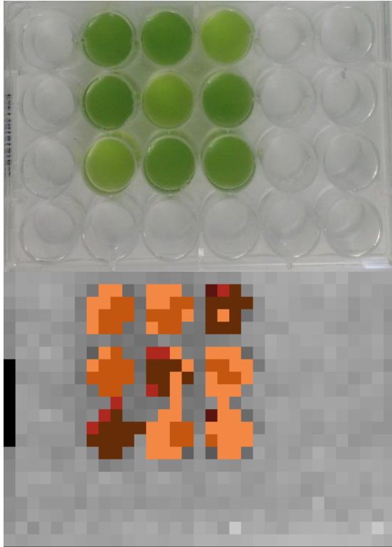
Figure 7. These pictures show the original pictures of the algae and the pictures of the algae after it has been analyzed. Wells D5, C4, and C3 have 16 PPT of salt. Wells C5, D3, and D4 have 24 PPT of salt. Wells B4 and B5 have 48 PPT of salt.
